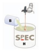
Empty the contents of the base component tin into the curing agent tin. To ensure that all of the base component is removed, the inside of the tin should be scraped. The material should then be mixed using a suitable slow
